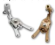
Bronze or aluminum cast point base for use on ridged roof, sloping or flat surfaces. Positive bolt tension cable clamping with four .187" diameter holes provided for nails or metal screws.
