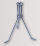
Galvanized steel tripod braces for additional support of long air terminals. Constructed of 1/4" mild steel with heavy section washer guides. All joints welded prior to galvanizing. Two .14" diameter mounting holes per leg furnished for installation. Suitable for 3/8", 1/2" and 5/8" diameter points.
