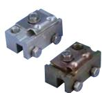
Bronze or aluminum machined point base for standing seam roofing systems. Bottom groove 1/2" wide by 3/4" deep to secure on seam with two set screws. Adjustable cable connector for conductor runs either parallel or perpendicular to the seam.
