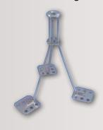
Galvanized steel tripod braces for additional support of long air terminals on flat or gently sloping surface when no penetration may be made for anchoring. Constructed of 1/4" mild steel with heavy section washer guides. All joints welded prior to galvanizing. For use with hot pitch, roofing compound or commercial adhesive on membrane surface or other locations. Suitable for 3/8", 1/2" and 5/8" diameter points.
