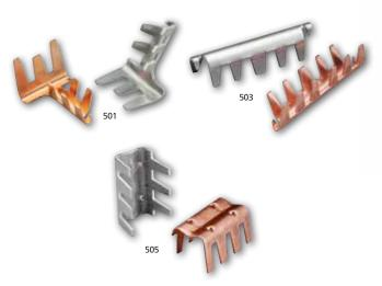
Copper or aluminum connector with compression type fingers to crimp over cable. Made from 14 gauge copper or 10 gauge aluminum sheet stock. For use on Class I structures only.
