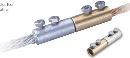
Machined aluminum bi-metallic connector for making connections between copper and aluminum cables in straight run. Two-bolt tension grip on each cable end. For use with all full size cables up to 4/0.
