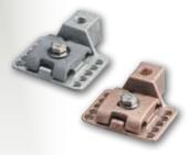
Bronze or aluminum cast adhesive point base for use on flat or vertical surfaces. Positive single bolt tension for multidirectional cable clamping. Four .250" diameter mounting holes for bolts or screws.
