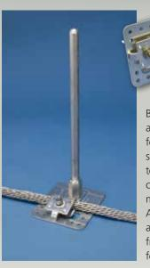
Bronze, tinned bronze or aluminum stamped adhesive base for use on flat, vertical or sloping surfaces. Positive single bolt tension for multi-directional cable clamping. Four .281" diameter mounting holes for bolts or screws. Air terminal support tab is field adjustable for any angle as shown from 0-90°, eliminating the need for swivel adaptors.
