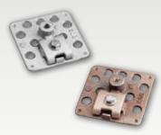
Bronze or aluminum cast adhesive point base for use on flat surfaces when no penetration may be made for anchoring. Positive single bolt tension cable clamping. For use with hot pitch, roofing compound or commercial adhesive on built-up roof surfaces or other locations.
