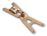
Bronze or aluminum cast point base for use on ridged roof, sloping or flat surfaces. May be easily formed. Positive bolt tension cable clamping with four .250" diameter holes provided for nails or metal screws.
