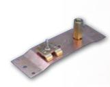
Copper or aluminum point base for use on narrow surface or roof edge. 8" long base with four .200" diameter holes for nails or screw anchors.
