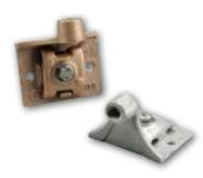
Bronze or aluminum cast point base for use on vertical surface with horizontal or vertical run of cable. Point attachment offset 2" from surface to clear overhang of wall cap or cover. Positive bolt tension cable clamping with two .281" diameter mounting holes for bolts or screws.
